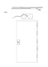
With the mounting plate secured to the wall and the whip in place proceed to the next step.
