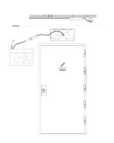
Connect the fixture to the whip with the provided connector. After the fixture is connected to the whip attach the fixture to the wall using the previously installed mounting plate.
