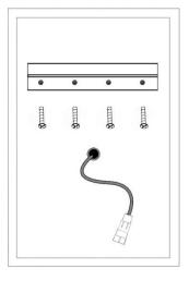
Attach the mirror mounting bracket to the wall using the appropriate screws. Ensure to not overtighten the screws so that you do not strip or snap the head off the screw.
